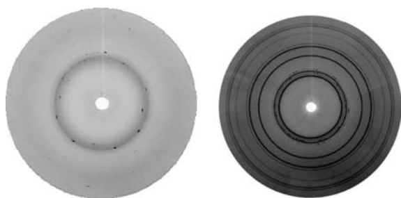
Figure 2. Diffraction plate image of nanocrystalline \text{Hf}_3\text{N}_4 at 12 GPa before laser heating (left) and crystallized tetragonal \text{Hf}_3\text{N}_4 after laser heating for 60 s (right). The heavily textured diffraction rings in both images are due to the nitrogen pressure transmitting medium/thermal insulator; these were removed by masking when the images were integrated.
